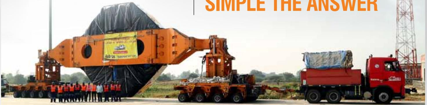
**END SHIELD** movement from L&T Hazira to RAPP, Rawatbhata using specially designed Rotatitting fixture to overcome en route bottlenecks
